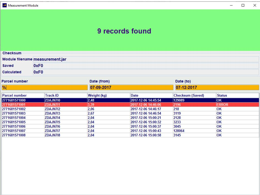
Figure (4) – Test screen of measurement module with search fields and result list (with ERROR entry)
